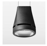
Suspended luminaire with LED, rated life of the LED L80/B10 > 50000 h, chromaticity tolerance 3 SDCM (initial), reflector with oval light distribution pattern, reflector pure aluminium 99,99% in MIRO-Silver®, canopy sheet steel, powder-coated, luminaire head die-cast aluminium, powder-coated, stratoblack
