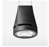
Suspended luminaire with LED, rated life of the LED L80/B10 > 50000 h, chromaticity tolerance 2 SDCM (initial), reflector with circular light distribution pattern, reflector pure aluminium 99,99% in MIRO-Silver®, canopy sheet steel, powder-coated, luminaire head die-cast aluminium, powder-coated, stratoblack
