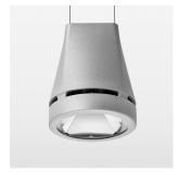
Suspended luminaire with LED, rated life of the LED L80/B10 > 50000 h, chromaticity tolerance 3 SDCM (initial), reflector with circular light distribution pattern, reflector pure aluminium 99,99% in MIRO-Silver®, canopy sheet steel, powder-coated, luminaire head die-cast aluminium, powder-coated, stratosilver
