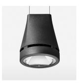
Suspended luminaire with LED, rated life of the LED L80/B10 > 50000 h, chromaticity tolerance 2 SDCM (initial), reflector with circular light distribution pattern, reflector pure aluminium 99,99% in MIRO-Silver®, canopy sheet steel, powder-coated, luminaire head die-cast aluminium, powder-coated, stratoblack
