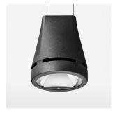
Suspended luminaire with LED, rated life of the LED L80/B10 > 50000 h, colour rendering index CRI > 80, chromaticity tolerance 2 SDCM (initial), reflector with circular light distribution pattern, reflector pure aluminium 99,99% in MIRO-Silver®, luminaire head die-cast aluminium, powder-coated, stratoblack, separate driver unit
