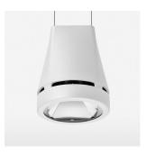
Suspended luminaire with LED, rated life of the LED L80/B10 > 50000 h, colour rendering index CRI > 90, chromaticity tolerance 2 SDCM (initial), reflector with circular light distribution pattern, reflector pure aluminium 99,99% in MIRO-Silver®, luminaire head die-cast aluminium, powder-coated, stratowhite, separate driver unit
