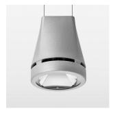
Suspended luminaire with LED, rated life of the LED L80/B10 > 50000 h, chromaticity tolerance 3 SDCM (initial), reflector with circular light distribution pattern, reflector pure aluminium 99,99% in MIRO-Silver®, luminaire head die-cast aluminium, powder-coated, stratosilver, separate driver
