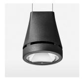
Suspended luminaire with LED, rated life of the LED L80/B10 > 50000 h, chromaticity tolerance 2 SDCM (initial), reflector with circular light distribution pattern, reflector pure aluminium 99,99% in MIRO-Silver®, luminaire head die-cast aluminium, powder-coated, stratoblack, separate driver unit
