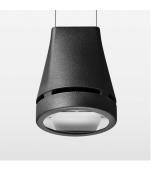
Suspended luminaire with LED, rated life of the LED L80/B10 > 50000 h, chromaticity tolerance 2 SDCM (initial), reflector with oval light distribution pattern, reflector pure aluminium 99,99% in MIRO-Silver®, luminaire head die-cast aluminium, powder-coated, stratoblack, separate driver unit
