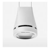
Suspended luminaire with LED, rated life of the LED L80/B10 > 50000 h, chromaticity tolerance 2 SDCM (initial), reflector with oval light distribution pattern, reflector pure aluminium 99,99% in MIRO-Silver®, luminaire head die-cast aluminium, powder-coated, stratowhite, separate driver unit
