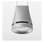
Suspended luminaire with LED, rated life of the LED L80/B10 > 50000 h, chromaticity tolerance 3 SDCM (initial), reflector with oval light distribution pattern, reflector pure aluminium 99,99% in MIRO-Silver®, luminaire head die-cast aluminium, powder-coated, stratosilver, separate driver unit
