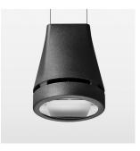
Suspended luminaire with LED, rated life of the LED L80/B10 > 50000 h, chromaticity tolerance 3 SDCM (initial), reflector with oval light distribution pattern, reflector pure aluminium 99,99% in MIRO-Silver®, luminaire head die-cast aluminium, powder-coated, stratoblack, separate driver unit
