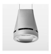
Suspended luminaire with LED, rated life of the LED L80/B10 > 50000 h, colour rendering index CRI > 90, chromaticity tolerance 2 SDCM (initial), reflector with oval light distribution pattern, reflector pure aluminium 99,99% in MIRO-Silver®, luminaire head die-cast aluminium, powder-coated, stratosilver, separate driver unit
