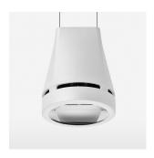
Suspended luminaire with LED, rated life of the LED L80/B10 > 50000 h, chromaticity tolerance 3 SDCM (initial), reflector with oval light distribution pattern, reflector pure aluminium 99,99% in MIRO-Silver®, luminaire head die-cast aluminium, powder-coated, stratowhite, separate driver unit
