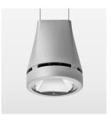
Suspended luminaire with LED, rated life of the LED L80/B10 > 50000 h, chromaticity tolerance 2 SDCM (initial), reflector with circular light distribution pattern, reflector pure aluminium 99,99% in MIRO-Silver®, luminaire head die-cast aluminium, powder-coated, stratosilver, separate driver unit
