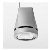
Suspended luminaire with LED, rated life of the LED L80/B10 > 50000 h, colour rendering index CRI > 90, chromaticity tolerance 2 SDCM (initial), reflector with circular light distribution pattern, reflector pure aluminium 99,99% in MIRO-Silver®, luminaire head die-cast aluminium, powder-coated, stratosilver, separate driver unit
