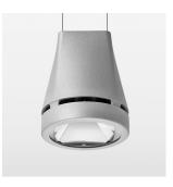
Suspended luminaire with LED, rated life of the LED L80/B10 > 50000 h, chromaticity tolerance 3 SDCM (initial), reflector with circular light distribution pattern, reflector pure aluminium 99,99% in MIRO-Silver®, luminaire head die-cast aluminium, powder-coated, stratosilver, separate driver unit
