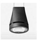
Suspended luminaire with LED, rated life of the LED L80/B10 > 50000 h, chromaticity tolerance 2 SDCM (initial), reflector with circular light distribution pattern, reflector pure aluminium 99,99% in MIRO-Silver®, luminaire head die-cast aluminium, powder-coated, stratoblack, separate driver unit
