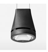
Suspended luminaire with LED, rated life of the LED L80/B10 > 50000 h, colour rendering index CRI > 90, chromaticity tolerance 2 SDCM (initial), reflector with circular light distribution pattern, reflector pure aluminium 99,99% in MIRO-Silver®, luminaire head die-cast aluminium, powder-coated, stratoblack, separate driver unit
