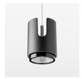
Suspended luminaire with LED, rated life of the LED L80/B10 > 50000 h, chromaticity tolerance 2 SDCM (initial), LED hybrid technology, 3D silicone lens to reduce the proportion of scattered light, reflector with circular light distribution pattern, reflector pure aluminium 99,99% in MIRO-Silver®, segmented and faceted, exchangeable reflector unit in high-sheen black plastic, with glass cover, luminaire housing die-cast aluminium, powder-coated, stratoblack, separate driver unit
