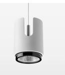
Suspended luminaire with LED, rated life of the LED L80/B10 > 50000 h, chromaticity tolerance 2 SDCM (initial), LED hybrid technology, 3D silicone lens to reduce the proportion of scattered light, reflector with circular light distribution pattern, reflector pure aluminium 99,99% in MIRO-Silver®, segmented and faceted, exchangeable reflector unit in high-sheen black plastic, with glass cover, luminaire housing die-cast aluminium, powder-coated, stratowhite, separate driver unit
