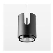
Suspended luminaire with LED, rated life of the LED L80/B10 > 50000 h, colour rendering index CRI > 90, chromaticity tolerance 2 SDCM (initial), , reflector with circular light distribution pattern, reflector pure aluminium 99,99% in MIRO-Silver®, segmented and faceted, exchangeable reflector unit in high-sheen black plastic, with glass cover, luminaire housing die-cast aluminium, powder-coated, stratoblack, separate driver unit
