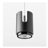
Suspended luminaire with LED, rated life of the LED L80/B10 > 50000 h, chromaticity tolerance 3 SDCM (initial), , reflector with circular light distribution pattern, reflector pure aluminium 99,99% in MIRO-Silver®, segmented and faceted, exchangeable reflector unit in high-sheen black plastic, with glass cover, luminaire housing die-cast aluminium, powder-coated, stratoblack, separate driver unit
