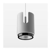
Suspended luminaire with LED, rated life of the LED L80/B10 > 50000 h, colour rendering index CRI > 80, chromaticity tolerance 2 SDCM (initial), LED hybrid technology, 3D silicone lens to reduce the proportion of scattered light, reflector with oval light distribution pattern, reflector pure aluminium 99,99% in MIRO-Silver®, segmented, exchangeable reflector unit in high-sheen black plastic, with glass cover, luminaire housing die-cast aluminium, powder-coated, stratosilver, separate driver unit
