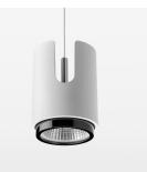
Suspended luminaire with LED, rated life of the LED L80/B10 > 50000 h, colour rendering index CRI > 80, chromaticity tolerance 2 SDCM (initial), LED hybrid technology, 3D silicone lens to reduce the proportion of scattered light, reflector with oval light distribution pattern, reflector pure aluminium 99,99% in MIRO-Silver®, segmented, exchangeable reflector unit in high-sheen black plastic, with glass cover, luminaire housing die-cast aluminium, powder-coated, stratowhite, separate driver unit
