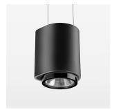
Suspended luminaire with LED, rated life of the LED L80/B10 > 50000 h, chromaticity tolerance 3 SDCM (initial), LED hybrid technology, 3D silicone lens to reduce the proportion of scattered light, reflector with circular light distribution pattern, reflector pure aluminium 99,99% in MIRO-Silver®, segmented and faceted, exchangeable reflector unit in high-sheen black plastic, with glass cover, luminaire housing die-cast aluminium, powder-coated, stratoblack, separate driver unit
