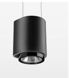
Suspended luminaire with LED, rated life of the LED L80/B10 > 50000 h, chromaticity tolerance 2 SDCM (initial), , reflector with circular light distribution pattern, reflector pure aluminium 99,99% in MIRO-Silver®, segmented and faceted, exchangeable reflector unit in high-sheen black plastic, with glass cover, luminaire housing die-cast aluminium, powder-coated, stratoblack, separate driver unit
