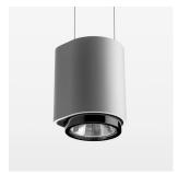
Suspended luminaire with LED, rated life of the LED L80/B10 > 50000 h, colour rendering index CRI > 96, chromaticity tolerance 3 SDCM (initial), , reflector with circular light distribution pattern, reflector pure aluminium 99,99% in MIRO-Silver®, segmented and faceted, exchangeable reflector unit in high-sheen black plastic, with glass cover, luminaire housing die-cast aluminium, powder-coated, stratosilver
