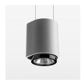
Suspended luminaire with LED, rated life of the LED L80/B10 > 50000 h, colour rendering index CRI > 90, chromaticity tolerance 2 SDCM (initial), , reflector with circular light distribution pattern, reflector pure aluminium 99,99% in MIRO-Silver®, segmented and faceted, exchangeable reflector unit in high-sheen black plastic, with glass cover, luminaire housing die-cast aluminium, powder-coated, stratosilver, separate driver unit
