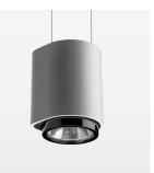
Suspended luminaire with LED, rated life of the LED L80/B10 > 50000 h, chromaticity tolerance 2 SDCM (initial), , reflector with circular light distribution pattern, reflector pure aluminium 99,99% in MIRO-Silver®, segmented and faceted, exchangeable reflector unit in high-sheen black plastic, with glass cover, luminaire housing die-cast aluminium, powder-coated, stratosilver, separate driver unit
