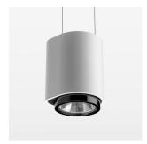
Suspended luminaire with LED, rated life of the LED L80/B10 > 50000 h, colour rendering index CRI > 80, chromaticity tolerance 2 SDCM (initial), , reflector with circular light distribution pattern, reflector pure aluminium 99,99% in MIRO-Silver®, segmented and faceted, exchangeable reflector unit in high-sheen black plastic, with glass cover, luminaire housing die-cast aluminium, powder-coated, stratowhite, separate driver unit
