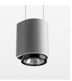
Suspended luminaire with LED, rated life of the LED L80/B10 > 50000 h, chromaticity tolerance 3 SDCM (initial), LED hybrid technology, 3D silicone lens to reduce the proportion of scattered light, reflector with oval light distribution pattern, reflector pure aluminium 99,99% in MIRO-Silver®, segmented, exchangeable reflector unit in high-sheen black plastic, with glass cover, luminaire housing die-cast aluminium, powder-coated, stratosilver, separate driver unit
