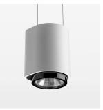
Suspended luminaire with LED, rated life of the LED L80/B10 > 50000 h, colour rendering index CRI > 80, chromaticity tolerance 2 SDCM (initial), LED hybrid technology, 3D silicone lens to reduce the proportion of scattered light, reflector with oval light distribution pattern, reflector pure aluminium 99,99% in MIRO-Silver®, segmented, exchangeable reflector unit in high-sheen black plastic, with glass cover, luminaire housing die-cast aluminium, powder-coated, stratowhite, separate driver unit
