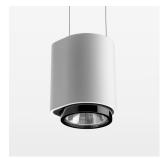
Suspended luminaire with LED, rated life of the LED L80/B10 > 50000 h, colour rendering index CRI > 80, chromaticity tolerance 2 SDCM (initial), LED hybrid technology, 3D silicone lens to reduce the proportion of scattered light, reflector with oval light distribution pattern, reflector pure aluminium 99,99% in MIRO-Silver®, segmented, exchangeable reflector unit in high-sheen black plastic, with glass cover, luminaire housing die-cast aluminium, powder-coated, stratowhite
