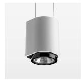
Suspended luminaire with LED, rated life of the LED L80/B10 > 50000 h, chromaticity tolerance 2 SDCM (initial), LED hybrid technology, 3D silicone lens to reduce the proportion of scattered light, reflector with oval light distribution pattern, reflector pure aluminium 99,99% in MIRO-Silver®, segmented, exchangeable reflector unit in high-sheen black plastic, with glass cover, luminaire housing die-cast aluminium, powder-coated, stratowhite
