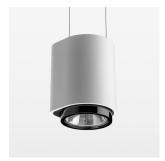
Suspended luminaire with LED, rated life of the LED L80/B10 > 50000 h, chromaticity tolerance 2 SDCM (initial), LED hybrid technology, 3D silicone lens to reduce the proportion of scattered light, reflector with oval light distribution pattern, reflector pure aluminium 99,99% in MIRO-Silver®, segmented, exchangeable reflector unit in high-sheen black plastic, with glass cover, luminaire housing die-cast aluminium, powder-coated, stratowhite
