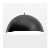
Decorative suspended luminaire with hub holder E27, max 150W, shade made of painted aluminium, black / pure white, metal trim ring (diameter 95mm) around hub holder, 28 ventilation openings (diameter 5mm) conzentric circular arrangement, double-isulated cabling, clampingdevice on cable ends if feed cable > 80 mm, power feed cable and canopy black, steel cable hanging set, ceiling-mounting, 1.5m cable
