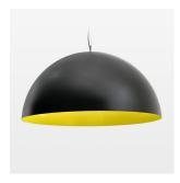
Decorative suspended luminaire with hub holder E27, max 150W, shade made of painted aluminium, black / traffic yellow, metal trim ring (diameter 95mm) around hub holder, 28 ventilation openings (diameter 5mm) conzentric circular arrangement, double-isulated cabling, clampingdevice on cable ends if feed cable > 80 mm, power feed cable and canopy black, steel cable hanging set, ceiling-mounting, 3m cable
