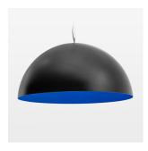
Decorative suspended luminaire with hub holder E27, max 150W, shade made of painted aluminium, black / traffic blue, metal trim ring (diameter 95mm) around hub holder, 28 ventilation openings (diameter 5mm) conzentric circular arrangement, double-isulated cabling, clampingdevice on cable ends if feed cable > 80 mm, power feed cable and canopy black, steel cable hanging set, ceiling-mounting, 3m cable
