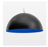
Decorative suspended luminaire with hub holder E27, max 150W, shade made of painted aluminium, black / traffic blue, metal trim ring (diameter 95mm) around hub holder, 28 ventilation openings (diameter 5mm) conzentric circular arrangement, double-isulated cabling, clampingdevice on cable ends if feed cable > 80 mm, power feed cable and canopy black, steel cable hanging set, ceiling-mounting, 6m cable
