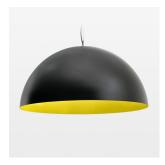
Decorative suspended luminaire with hub holder E27, max 150W, shade made of painted aluminium, black / traffic yellow, metal trim ring (diameter 95mm) around hub holder, 28 ventilation openings (diameter 5mm) conzentric circular arrangement, double-isulated cabling, clampingdevice on cable ends if feed cable > 80 mm, power feed cable and canopy black, steel cable hanging set, multiadapter, 1.5m cable
