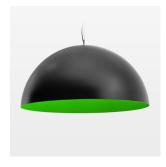
Decorative suspended luminaire with hub holder E27, max 150W, shade made of painted aluminium, black / yellow-green, metal trim ring (diameter 95mm) around hub holder, 28 ventilation openings (diameter 5mm) conzentric circular arrangement, double-isulated cabling, clampingdevice on cable ends if feed cable > 80 mm, power feed cable and canopy black, steel cable hanging set, multiadapter, 1.5m cable
