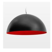
Decorative suspended luminaire with hub holder E27, max 150W, shade made of painted aluminium, black / traffic red, metal trim ring (diameter 95mm) around hub holder, 28 ventilation openings (diameter 5mm) conzentric circular arrangement, double-isulated cabling, clampingdevice on cable ends if feed cable > 80 mm, power feed cable and canopy black, steel cable hanging set, multiadapter, 1.5m cable
