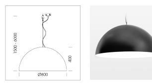
Decorative suspended luminaire with hub holder E27, max 150W, shade made of painted aluminium, black / pure white, metal trim ring (diameter 95mm) around hub holder, 28 ventilation openings (diameter 5mm) conzentric circular arrangement, double-isulated cabling, clampingdevice on cable ends if feed cable > 80 mm, power feed cable and canopy black, steel cable hanging set, multiadapter, 1.5m cable
