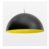
Decorative suspended luminaire with hub holder E27, max 150W, shade made of painted aluminium, black / traffic yellow, metal trim ring (diameter 95mm) around hub holder, 28 ventilation openings (diameter 5mm) conzentric circular arrangement, double-isulated cabling, clampingdevice on cable ends if feed cable > 80 mm, power feed cable and canopy black, steel cable hanging set, multiadapter, 3m cable
