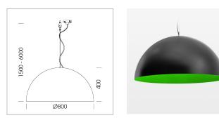
Decorative suspended luminaire with hub holder E27, max 150W, shade made of painted aluminium, black / yellow-green, metal trim ring (diameter 95mm) around hub holder, 28 ventilation openings (diameter 5mm) conzentric circular arrangement, double-isulated cabling, clampingdevice on cable ends if feed cable > 80 mm, power feed cable and canopy black, steel cable hanging set, multiadapter, 3m cable
