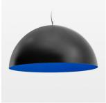
Decorative suspended luminaire with hub holder E27, max 150W, shade made of painted aluminium, black / traffic blue, metal trim ring (diameter 95mm) around hub holder, 28 ventilation openings (diameter 5mm) conzentric circular arrangement, double-isulated cabling, clampingdevice on cable ends if feed cable > 80 mm, power feed cable and canopy black, steel cable hanging set, multiadapter, 6m cable
