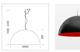
Decorative suspended luminaire with hub holder E27, max 150W, shade made of painted aluminium, black / traffic red, metal trim ring (diameter 95mm) around hub holder, 28 ventilation openings (diameter 5mm) conzentric circular arrangement, double-isulated cabling, clampingdevice on cable ends if feed cable > 80 mm, power feed cable and canopy black, steel cable hanging set, multiadapter, 6m cable
