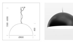
Decorative suspended luminaire with hub holder E27, max 150W, shade made of painted aluminium, black / pure white, metal trim ring (diameter 95mm) around hub holder, 28 ventilation openings (diameter 5mm) conzentric circular arrangement, double-isulated cabling, clampingdevice on cable ends if feed cable > 80 mm, power feed cable and canopy black, steel cable hanging set, multiadapter, 6m cable
