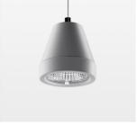
Suspended luminaire with LED, rated life of the LED L80/B10 > 50000 h, colour rendering index CRI > 80, chromaticity tolerance 3 SDCM (initial), rotation-symmetrical reflector with circular light distribution pattern, reflector pure aluminium 99,99% in MIRO-Silver®,segmented and faceted, 3D lens silicon to reduce the proportion of scattered light, luminaire head die-cast aluminium, powder-coated, stratosilver
